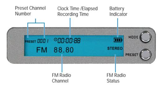
There are two other modes in Radio mode, FM Preset and FM Tuning mode. In FM Preset mode, you can select an FM preset channel. In FM Tuning mode, you can assign a preset to an FM channel. See "Using the Dell DJ Inline FM Tuner" for more information.
