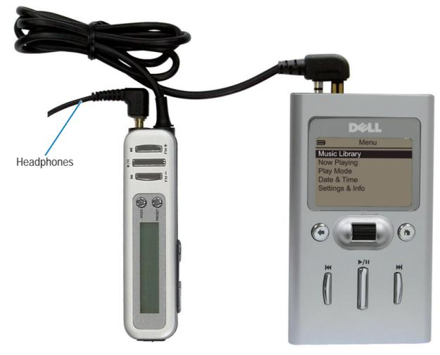
Connect ONLY the supplied Inline FM Tuner (part number F7492) or wired remote (part number F7495) to your Dell DJ player. Connecting other Inline FM Tuners or wired remotes to your Dell DJ player may cause permanent damage.
